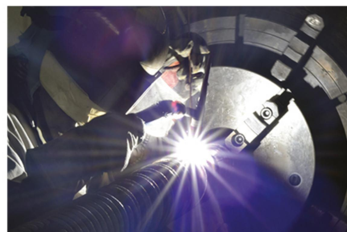
A weared screw can gives several problems such as poor quality of melt, poor flow. In such cases it may be convenient, instead of replacing it with a new one, to repair it. This operation is possible in most cases and leads to very advantageous results.
