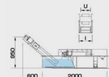
NV4 - NV5 - NV6 Nastro vasca particolari galleggianti Conveyor with cooling tank for floating parts
